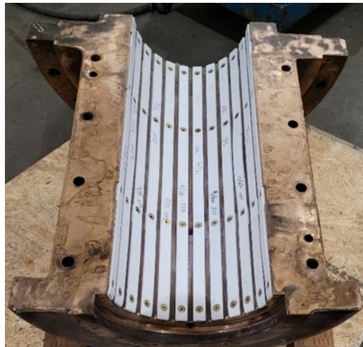
Fig 2: Lower guide bearing disassembled
